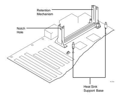
Push the Heat Sink Support Base onto the mainboard, until you hear a click sound. Check for a perfect fit.
